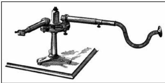
Figure 1: The original spectrophone designed by A.G. Bell.
