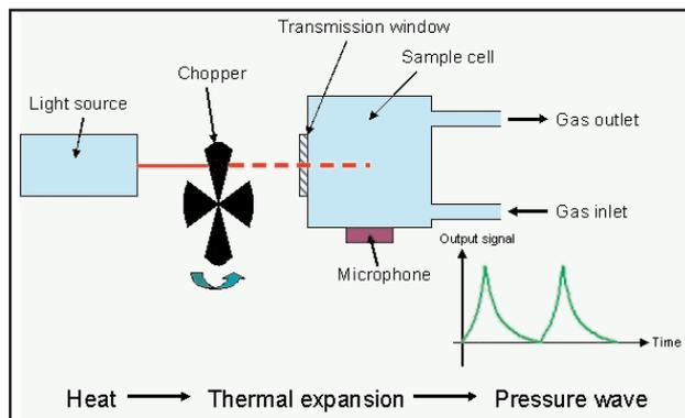
Figure 2: A basic photoacoustic gas detector.
